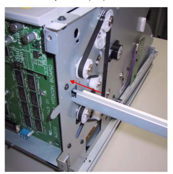
7. Insert it firmly to the back, and fix it with 1 screw (M3x6).
