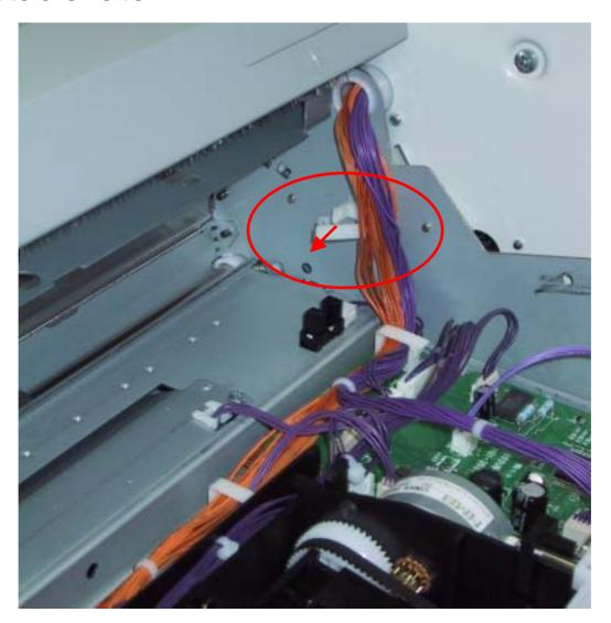
9. Insert the IP shaft to the hole of left side of main body's interior. (Insert the one that a tip is long.)
